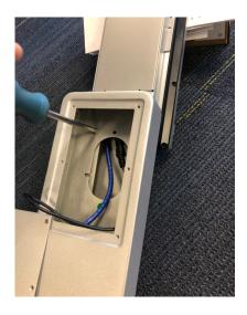
8. Replace all back panels by using the kiosk back cover screws (20).
